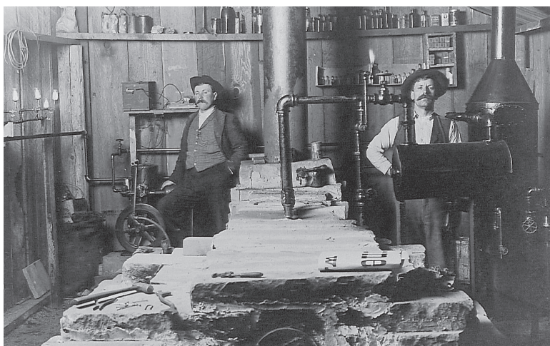
William McArthur (left), his brother, Robert McArthur, and William McArthur's patented retort for making illuminating gas out of Tenino coal. Note the row of lighted gas jets to the left of the photo. (Author's Collection)
